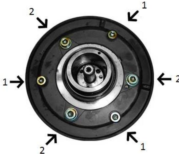
There are 2 bolt sizes that hold the AVCS sprocket together. Below are their tightening torques.
